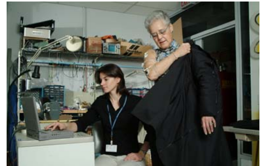
Postdoctoral research fellow, Brandi Row, uses electromyography (muscle activity recordings) with a research subject to assess whether the novel design features embedded in the winter coat prototype serve to reduce the physical challenge of donning and fastening a coat.
