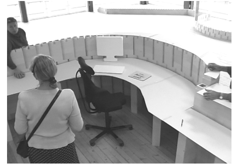
Figure 2: A model made in the Full Scale Laboratory using large plastic bricks and cardboard.
